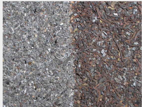
Metals and minerals for recycling recovered from bottom ash
