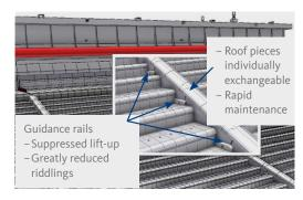
The rollers on which the carriage moves are now even longer-lasting and feature a hood for protection from deposits of ash and molten aluminium. The roof elements can also be replaced individually. Special guidance rails prevent parasitic air from entering.
