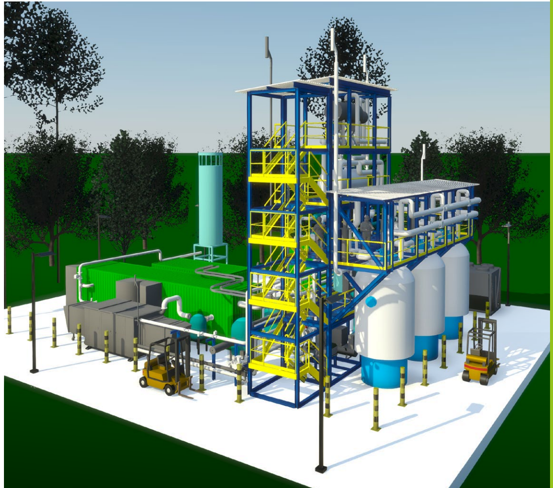
Pythia6000: HZI's catalytic methanation reactor series for 6,000 Nm 3 /h feed gas
