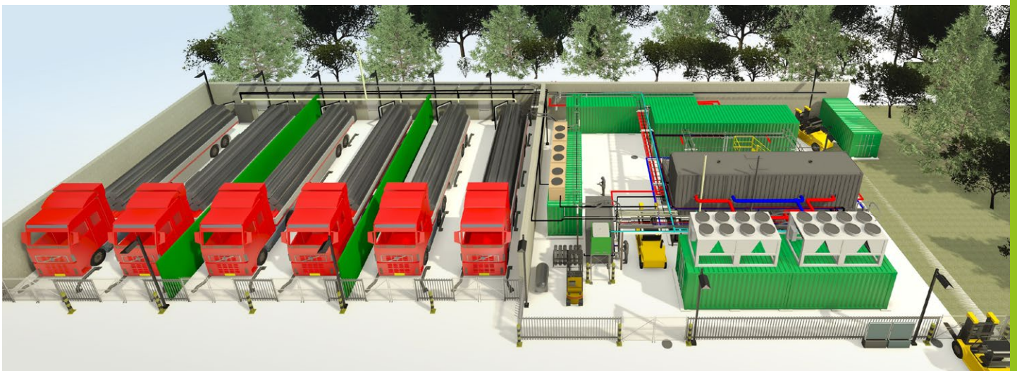
Illustration of HZI turnkey solution – plant under construction – including electrolyser (550 Nm 3 /h), compression, storage and distributed via tube trailers. Compact small-scale plant for commercial operation.
