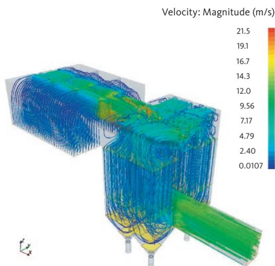
CFD Modelling of XEROSORP+: Bag filter, ammonia injection zone and SCR DeNOx
